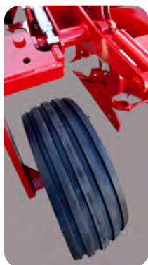
Bagmonteret dybde-trans- porthjul 250/65x14,5-12pr.
