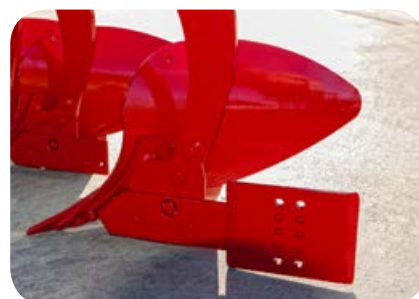
Landside extension, for better plough stability
