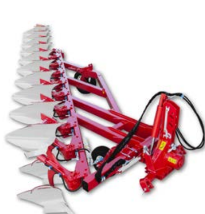
Reversible mounted shallow plough. From 5 up to 11 furrows Mini-NF/NH
