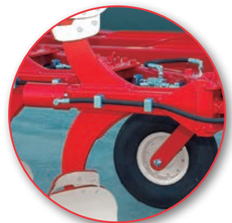
Hydraulic release system. Mini-HF, Mini-NH and Mini-SH
