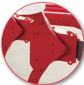
Shear bolt stone protection. Mini-NF and Mini-SF
