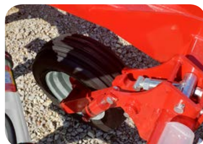
Front depth control wheel available as 6.00*9", 200/60 14,5" and 250/65 14,5" (depending on models)
